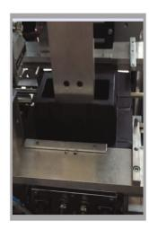
The carton, picked from side buffer, is preformed and folded during the down movement toward the main belt chain.
