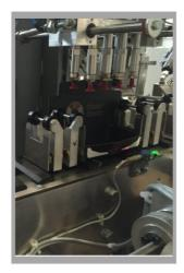
When the box is filled, the carton is glued and closed on sides during the chain movement toward exit zone.
