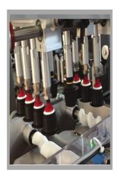
Just twisted (only the row needed by format) and separated, the Pick&Place picks up the cups and releases them inside the preformed box.
