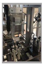
During the upper movement toward the exit belt, the carton is folded, glued and completely closed.
